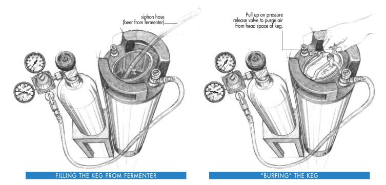
You can leave the gas tubing attached to the regulator for future use.
