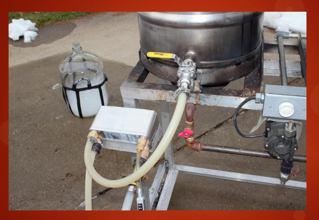
40 plate counterflow chiller set-up, with a Blichmann thrumometer
