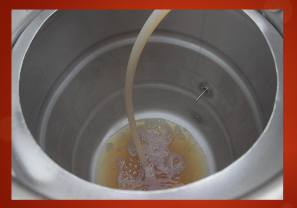
Splitting ½ of the wort to the hot liquor tank so I can aerate pre boil.
