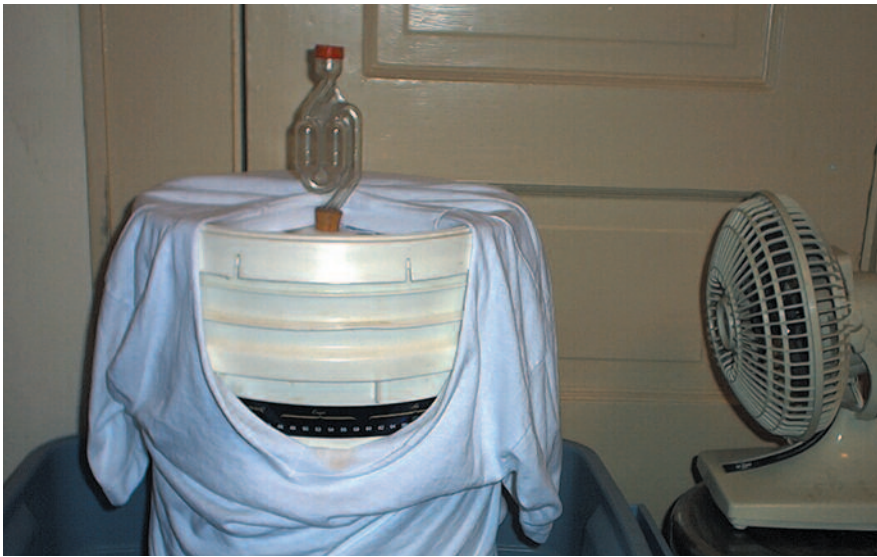
Plastic bucket fermenter in water bath with T-shirt and small fan blowing on bucket bath.
