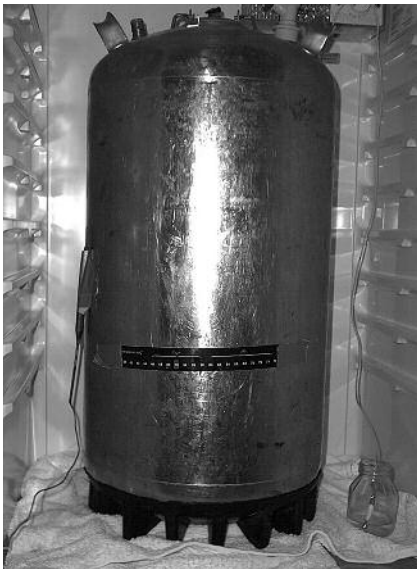
Cornelius keg fermenter in fridge with a liquid crystal thermometer strip and temperature sensor probe both affixed to fermenter with duct tape. (Note second probe for external thermometer in small water bath on right side of picture. This is so I can see what the ambient temperature is without having to open the fridge door.)
