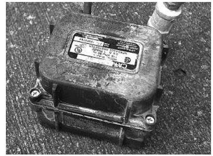
Submersible pump (Little Giant, model P-AAA) used in photo at bottom left.
